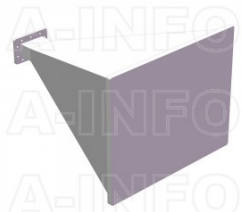
LB-284-20-ASPO Standard Gain Horn Antenna 2.6-3.95GHz 20dB Gain Rectangular Waveguide Interface
